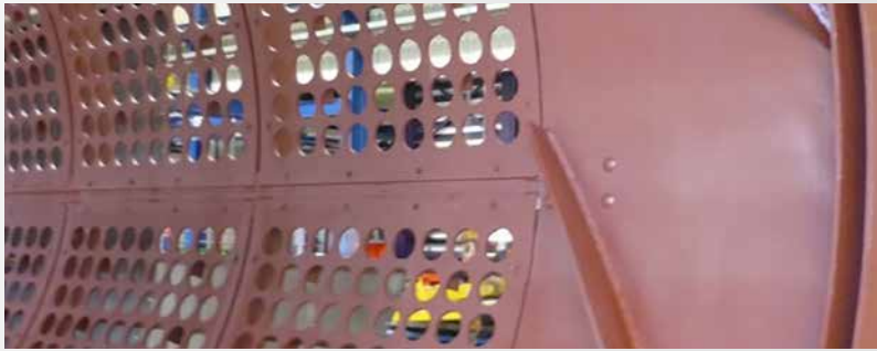
Infed of the drum without holes and labyrinth seal
