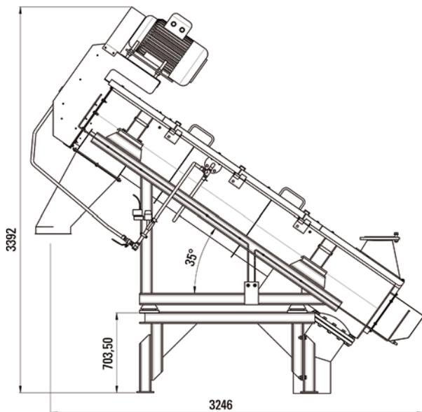
Fig. 3: Friction Washer series FA 3000
