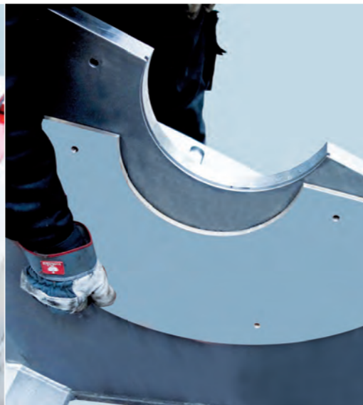
Exchangeable armor-plating of the housing
