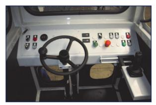
The GT can be easily moved by joystick and steering wheel
