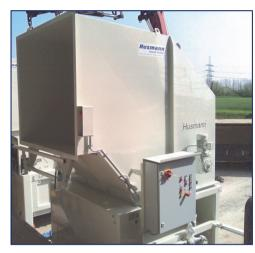
HSP-EL-V with feeding device and hopper suitable for loading bay operation
