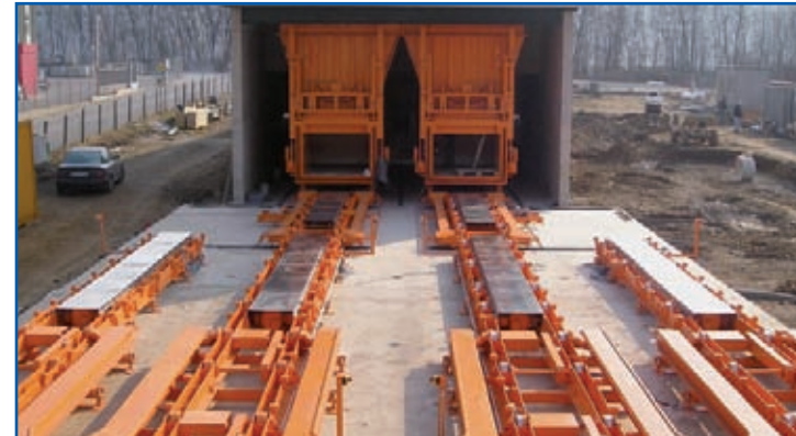
2 x MP 6000 in parallel operation with roller conveyor as container replacing device
