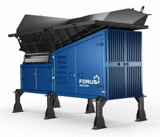
The FORUS **SES 250** is a two-shaft shredder with electric drive. It is used as a pre-shredder for different types of material. It shreds household waste, bulky waste, commercial waste, old wood and demolition wood, green cuttings and organic waste effortlessly. The slow-running shredder processes foils, paper and electric waste with equal efficiency. The final particle size varies from 150 to 350 mm, depending on the tools that are used.
