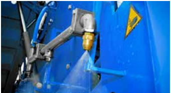
Concentrate injection for process optimization – for fast composting
