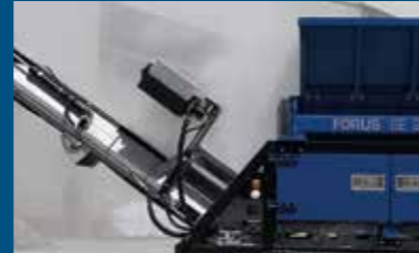
Hydraulically height-adjustable neodymium magnetic separator
