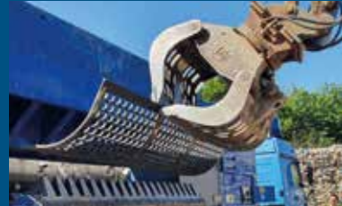
TEUTON: Screening basket system - to create a finished final grain size
