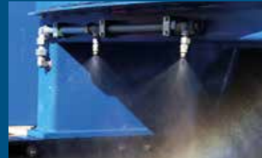
Material moistening device - for dust containment
